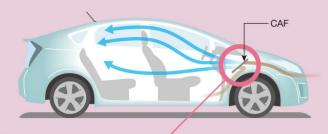
Just like with a household air-conditioner, a car's air-conditioner also has an air filter attached to it. It's called a Cabin Air Filter (CAF).
